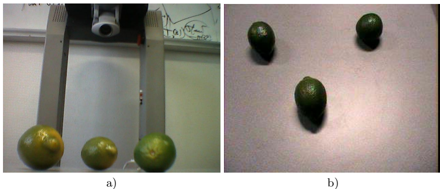
Fig. 3. Experimental environment: a) the PeopleBot is placed in front of a table with three green lemons. b) The image grabbed by the camera
