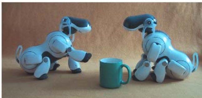
Fig. 1. An example of pointing shown with two robots. The robot on the left represents the adult who is pointing, the robot on the right represents the child who is learning to interpret the pointing gesture
